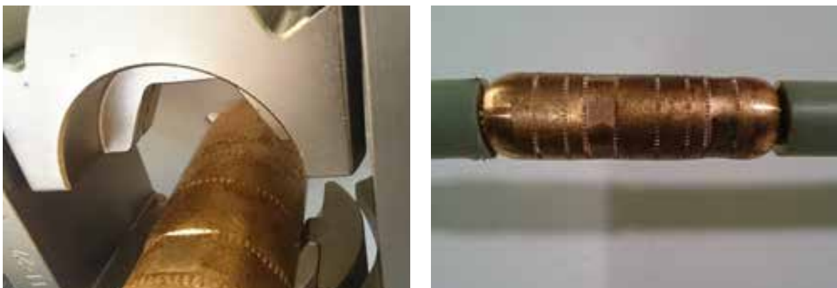
Figure 34 – Hexagonal compression die and copper connector (for stranded copper conductor) showing first compression position
