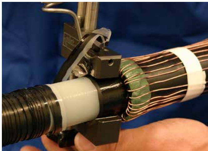
Figure 25 – This cutting tool creates a tapered screen edge at the selected position
