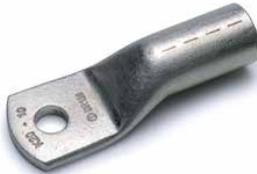
Figure 35 – Compression lug showing guide marks for hexagonal compression tool positions
