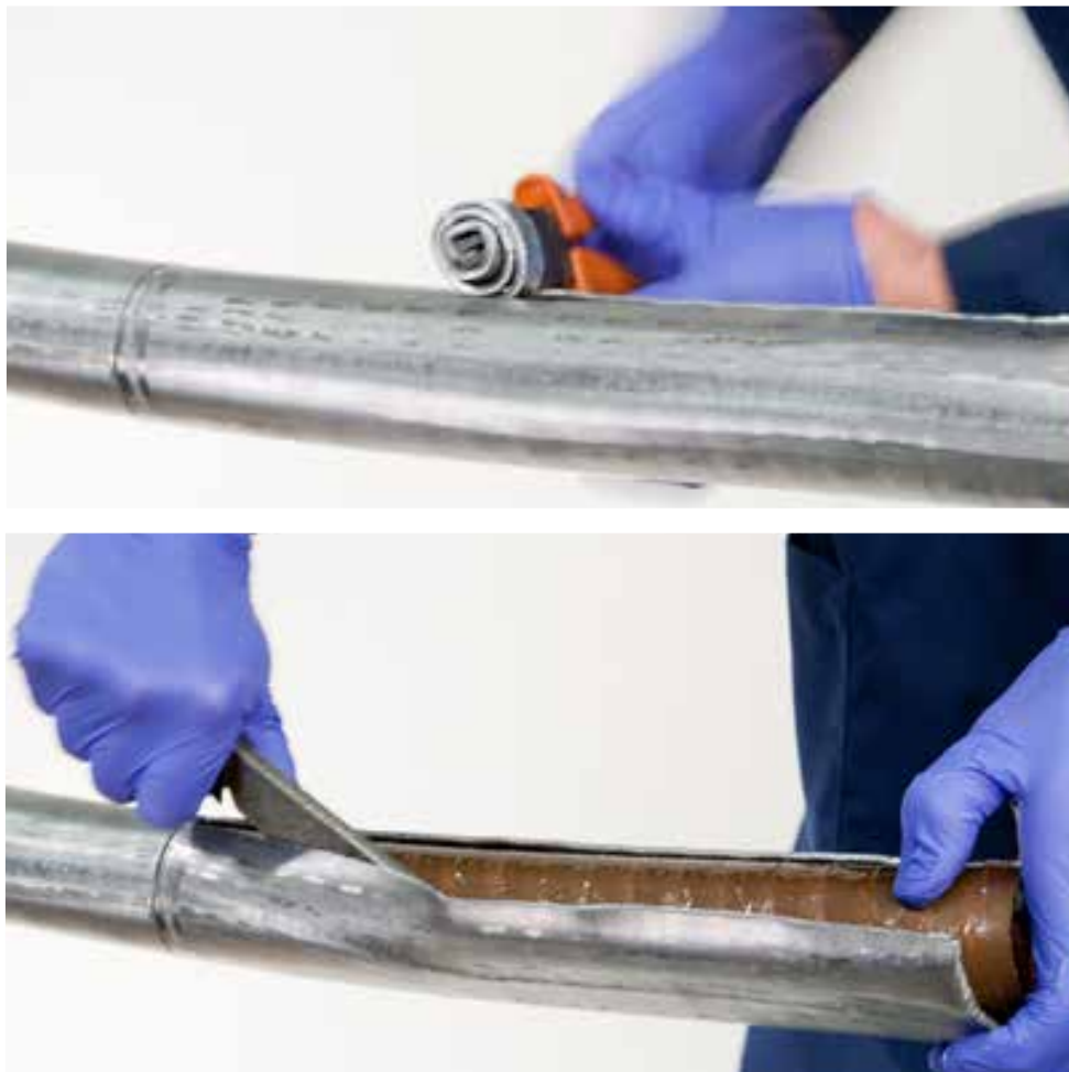
Figure 33 – A technique for removing lead sheaths
