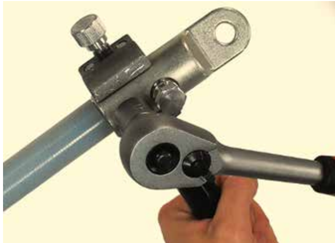
Figure 42 – Use of a support tool for installation of a shear-head mechanical lug
