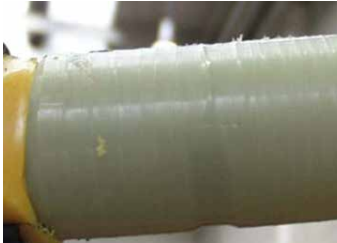
Figure 30 – Extremely rough insulation surface resulting from incorrect setting and/or misuse of screen removal tool
