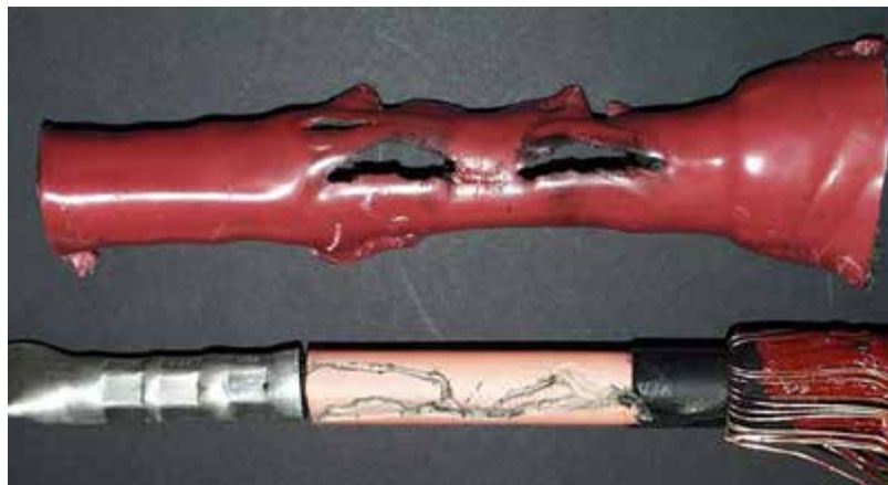
Figure 49 – Failure of a termination due to electrical tracking on the insulation surface
