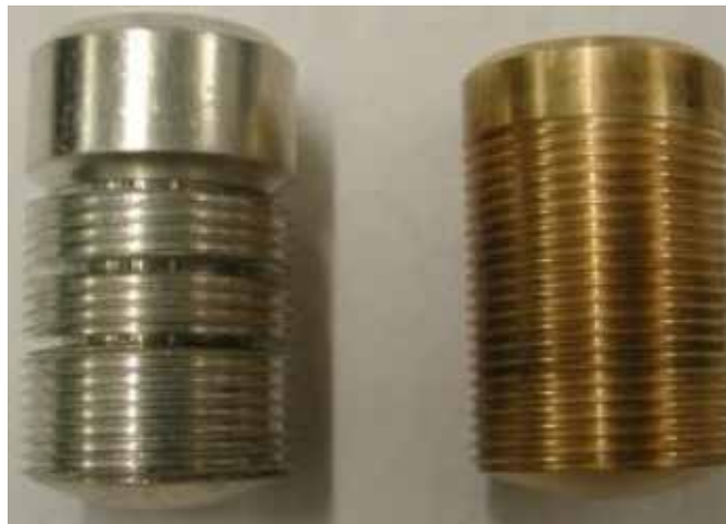
Figure 40 – Multi-shear position (left) and step-less shear (right) screws
