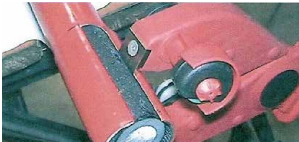
Figure 17 – Sheath removal tool for cables with aluminium laminate sheaths
