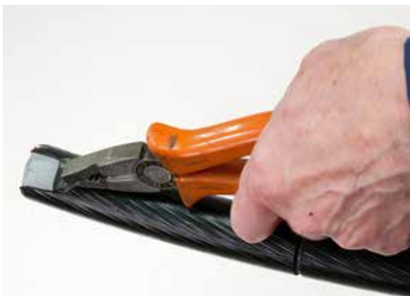
Figure 21 – Peeling strips of screen
