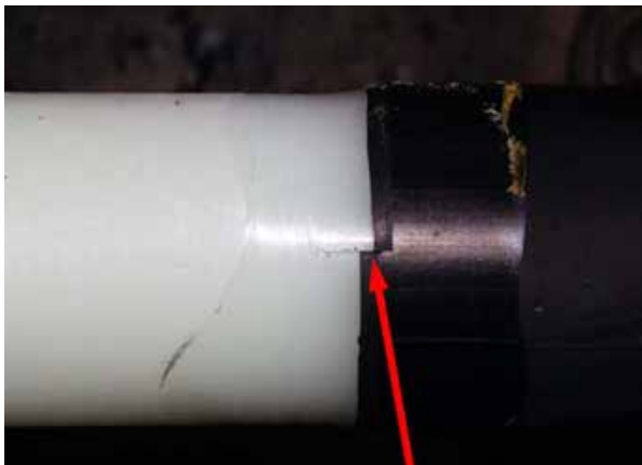
Figure 27 – Irregular conductive screen edge caused by incorrect use of the removal tool
